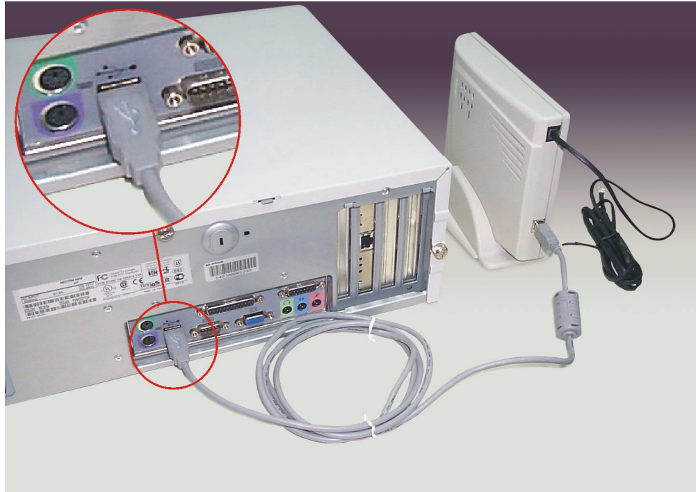
Figure 16: Cabling the jetSpeed 100 to the PC
