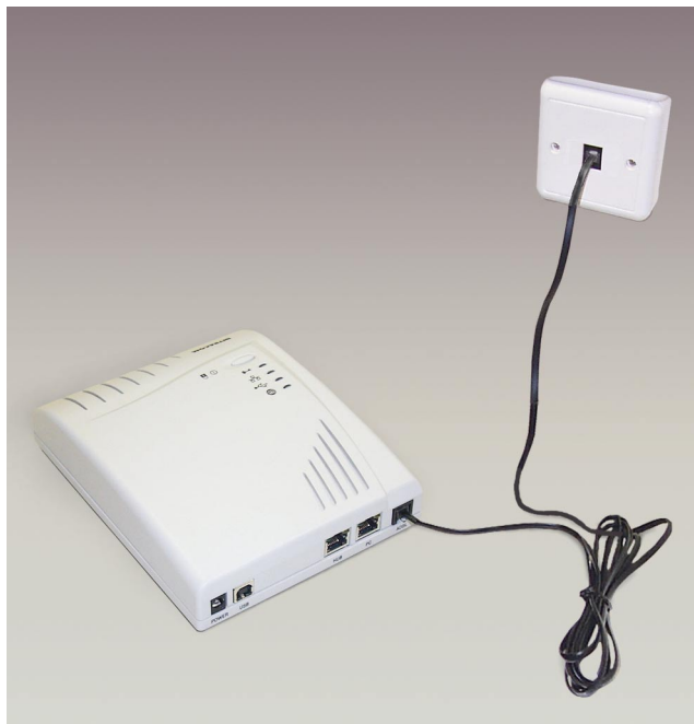
Figure 18: Connecting jetSpeed 500/500i to the ADSL line
