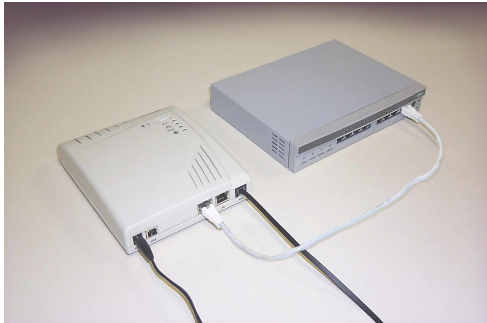
Figure 21: Connecting jetSpeed 500/500i to an Ethernet LAN
